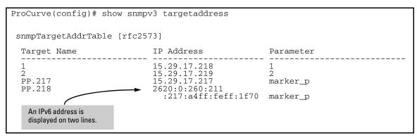
Figure 5-9. "show snmpv3 targetaddress" Command Output with IPv6 Address
